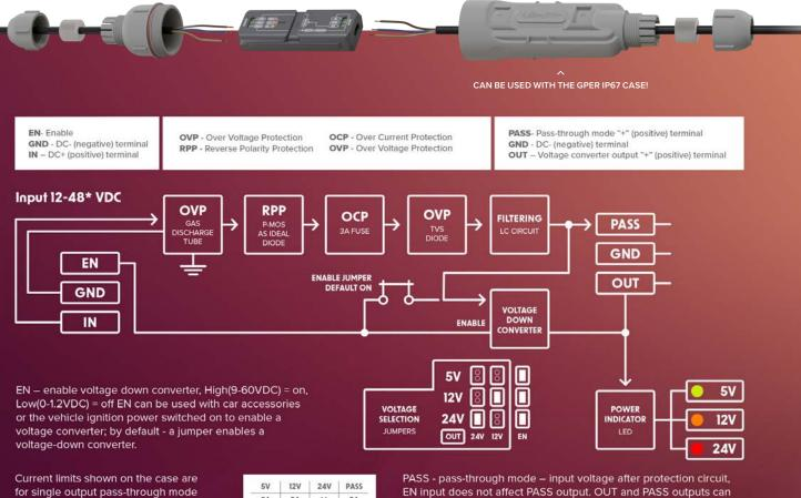
for single output pass-through mode or regulated 5/12/24V mode, but not for both outputs simultaneously.
