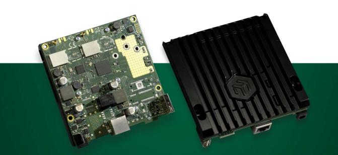
The powerful Wi-Fi 6 radio with MMCX connectors enables further customization: add a HGO-antenna-OUT and you've got yourself an excellent omnidirectional AP... or try the mANT30 PA antenna to create a powerful long-range point-to-point link!
